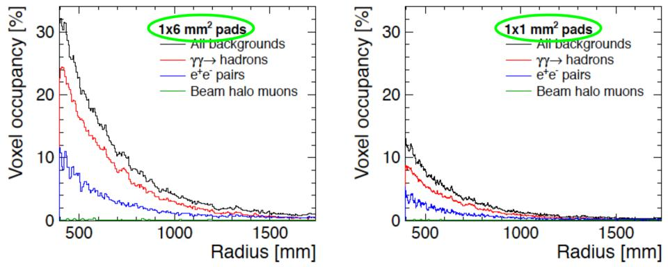
Plots are for Gas Electron Multiplier (GEM) + Pad readout, voxels of 25 ns
