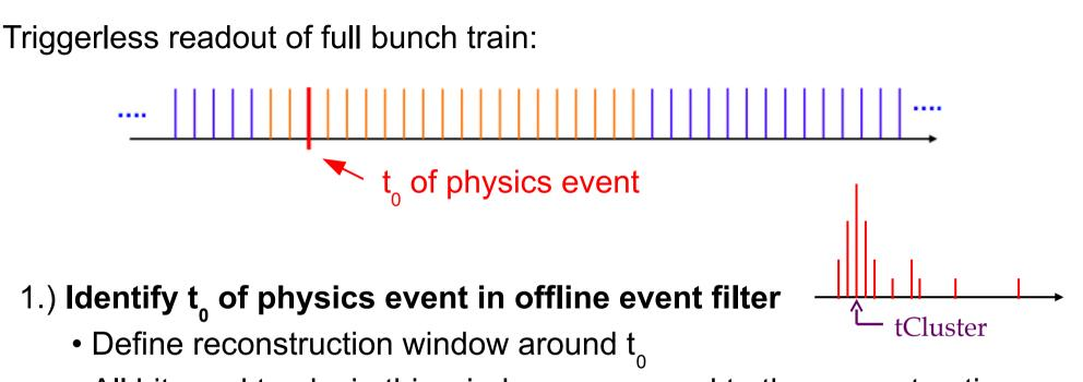
• All hits and tracks in this window are passed to the reconstruction  $\rightarrow$  Physics objects with precise p<sub>+</sub> and cluster time information
