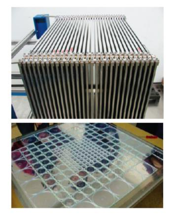
Scintillator tiles 3x3 cm<sup>2</sup> Read out by SiPM Data taken 2010/11 at CERN-PS/SPS, mixed beams 1-300 GeV
