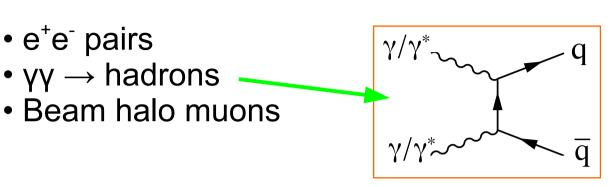
Coherent  $e^+e^-$  pairs: 7 · 10<sup>8</sup> per BX, very forward Incoherent  $e^+e^-$  pairs: 3 · 10<sup>5</sup> per BX, rather forward  $\rightarrow$  Detector design issue (high occupancies)
