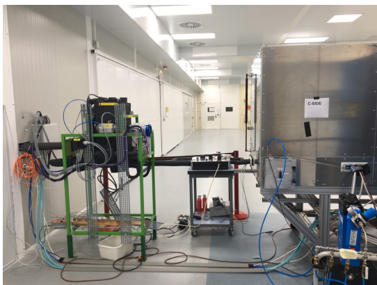
CO 2 plant with ~1.4 kW at -30°C
