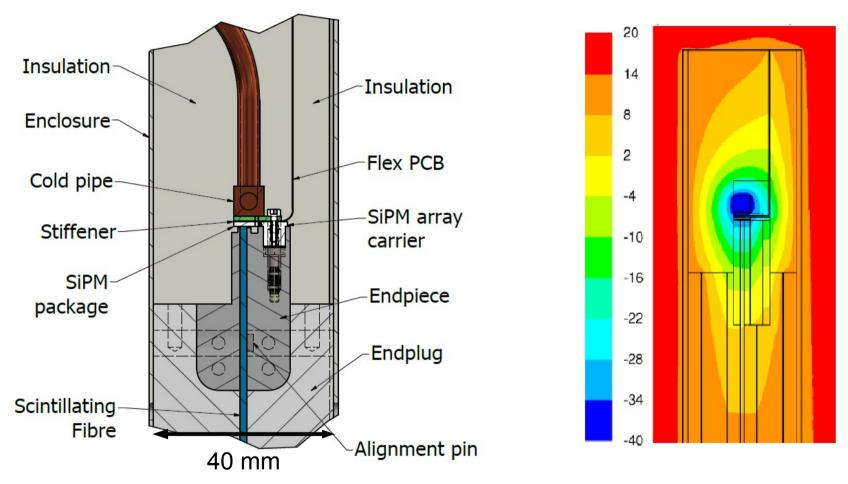
• Acceptable cluster rates require -40C cooling and +40C annealing
