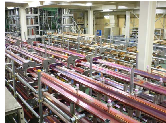
beam pipes after baking and TiN coating. They are temporary stocked until moved to tunnel
