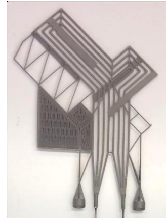
3d printed Titanium substrates, already prototyped for Upgrade I
