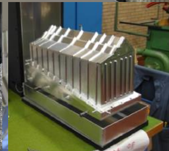
Internal mould support during machining steps
