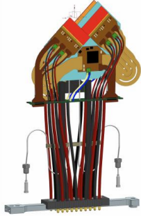
wire bonding and HV/LV/data cable attachment
