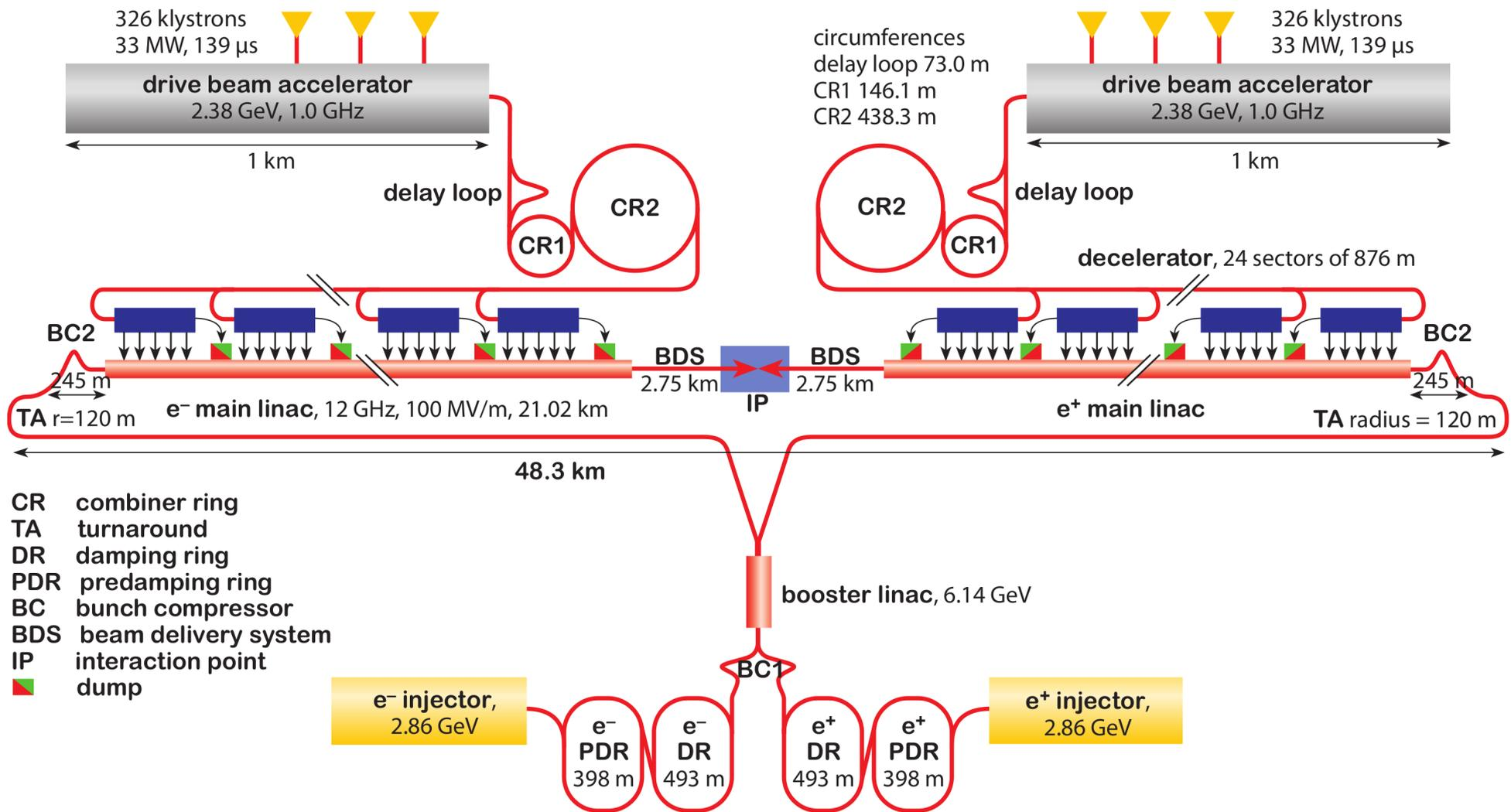
CLIC provides the potential for e<sup>+</sup>e<sup>-</sup> collisions up to  $\sqrt{s} = 3$  TeV:
