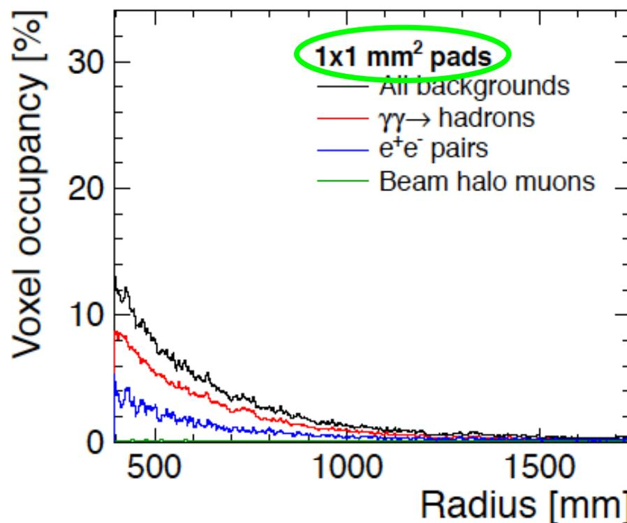
Plots are for Gas Electron Multiplier (GEM) + Pad readout, voxels of 25 ns
