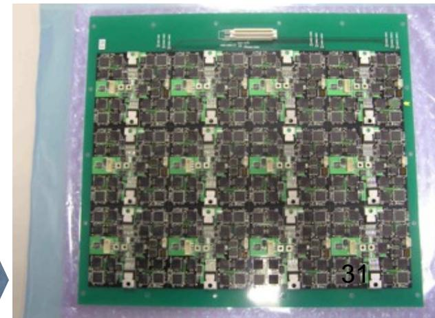
A test module as heat load with dummy heat-load FPGAs in place of S-ALTRO64.
