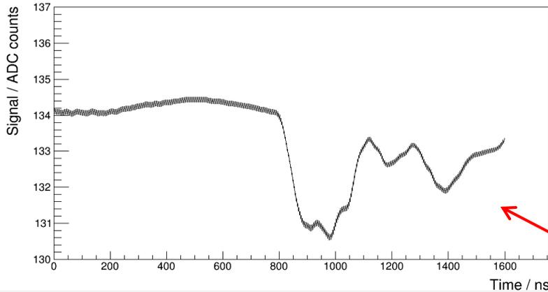
Large pick-up of telescope trigger
