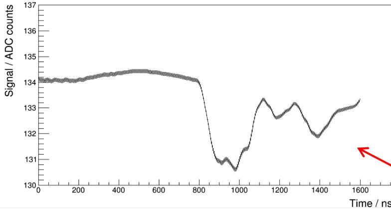
Large pick-up of telescope trigger
