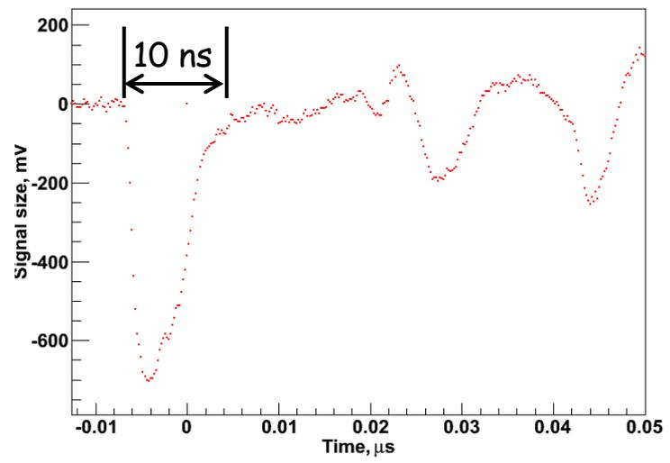
Analog signal from sapphire sensor
