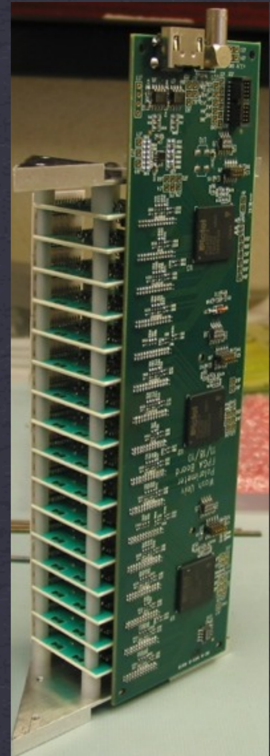
Tower with 8 detectors:
