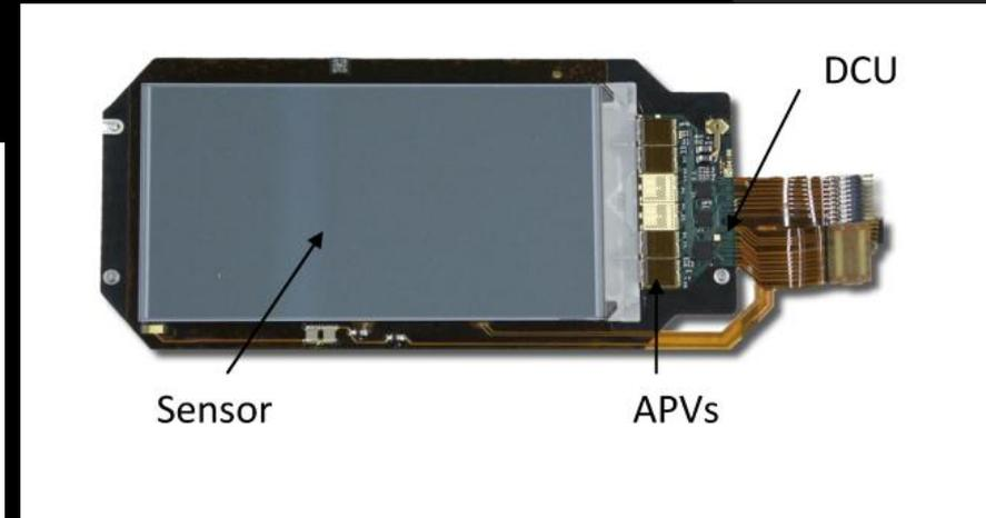
The detector control unit is a ASIC sitting on each of the tracker modules, with the ability to measure the temperature of the module as well as the leakage current and LV voltages applied.
