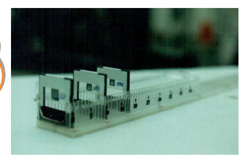
Yes, true, the neutron dose was probably a little off. But then, the radiation meter wouldn't show anywhere nearly as crazy numbers as for the old Aluminum sample holder, with all its bolts and nuts.
