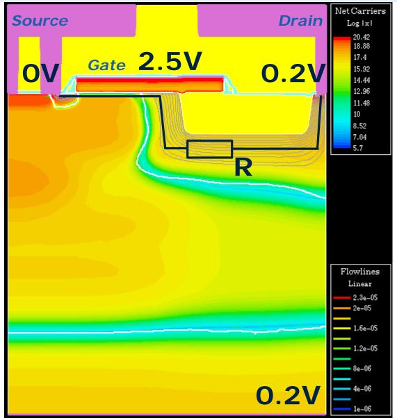
The on-state resistance is determined by the doping in the drain extension.
