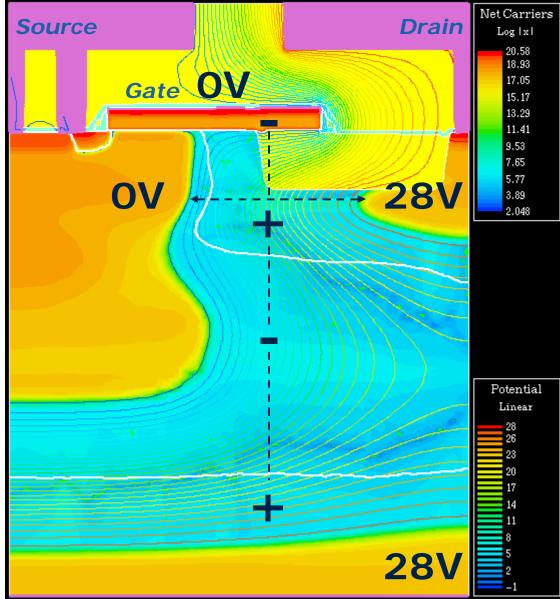
However, high doping in the drain extension limits the breakdown voltage!
