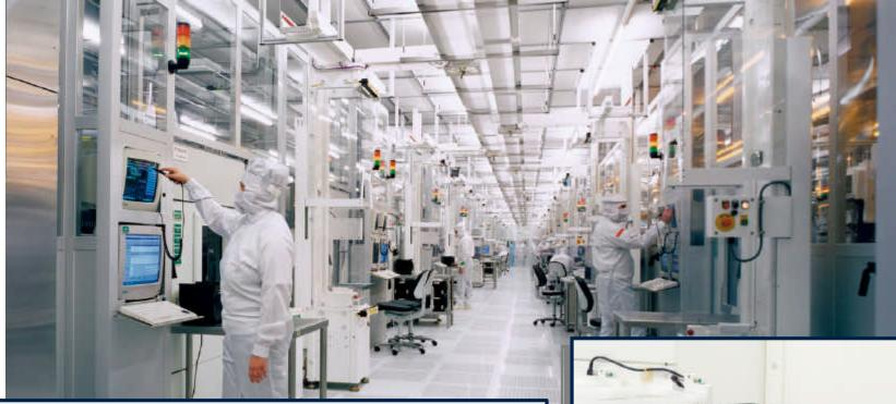
State-of-the-art semiconductor processing line for large-scale integration of electronic circuits on 200 mm silicon wafers
