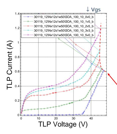
Transmission-line pulsing (TLP) is typically a 100-ns square-wave pulsed IV characterization. This is a good indication of device behavior under ESD stress.
