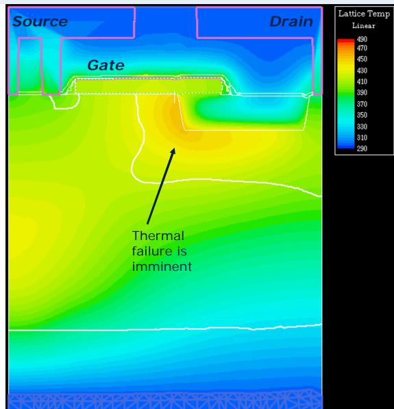
Electro-thermal TCAD simulations are quite helpful for optimizing the device robustness.
