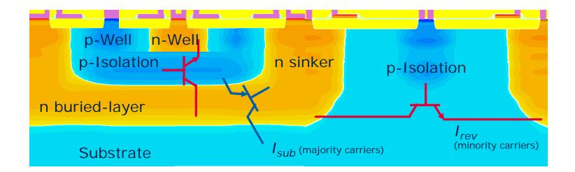
Power switching can introduce significant substrate noise, especially if inductive loads are driven
