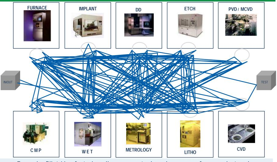
Example: Pilot-Line featuring all necessary tools and processes for a product cycle
