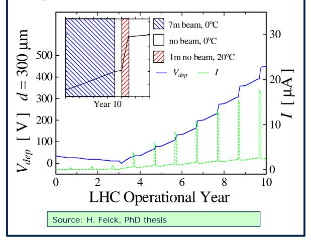
Our efforts to predict the operating lifetime of silicon detectors in the LHC experiments clearly addressed the customer's need for a solid decision basis in planning the overall experiment.
