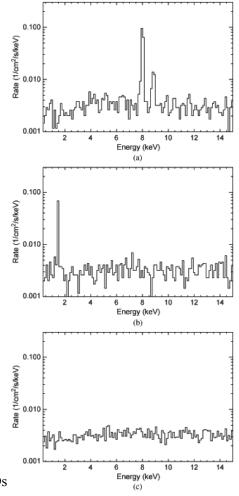
Fig. 12. A comparison of the fluorescence background due to ionization by cosmic-ray protons in an L2 orbit for three different graded Z shield designs for the eROSITA X-ray detectors. (a) Cu shield; (b) Cu-Al shield; (c)  $Cu - Al - B_4C$  shield.
