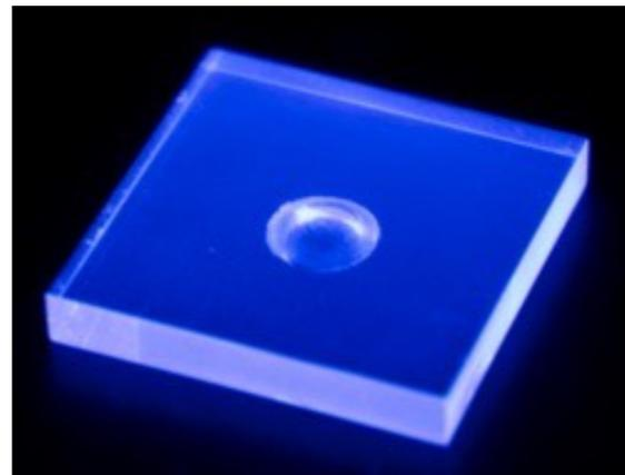
SiPMs in surface-mount packages for pick-and-place machines, together with fiberless tiles, pave the way towards automatic assembly of active layers
