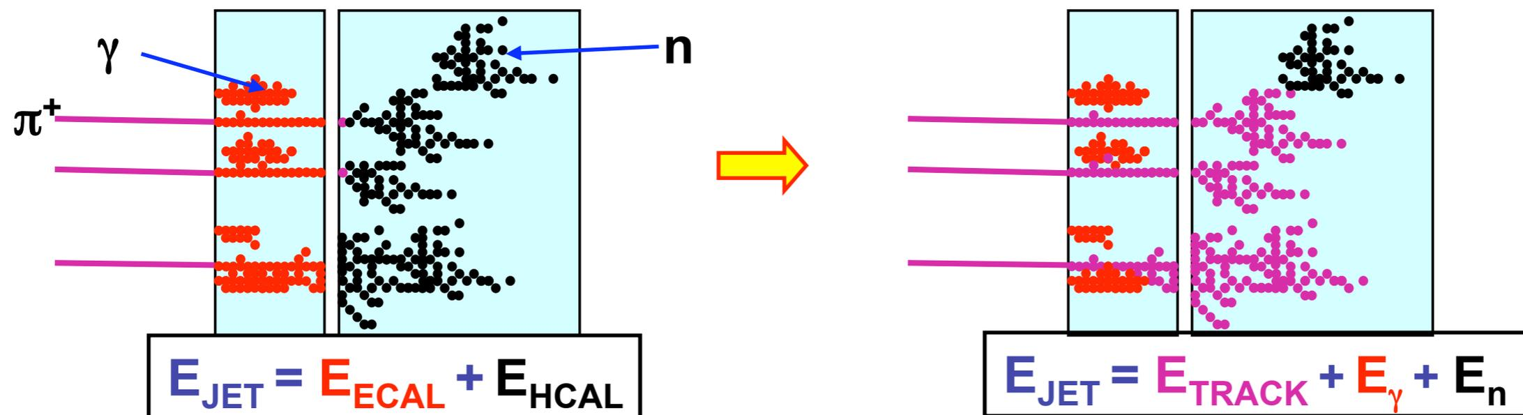
For best results: high granularity in the calorimeters to correctly separate showers
