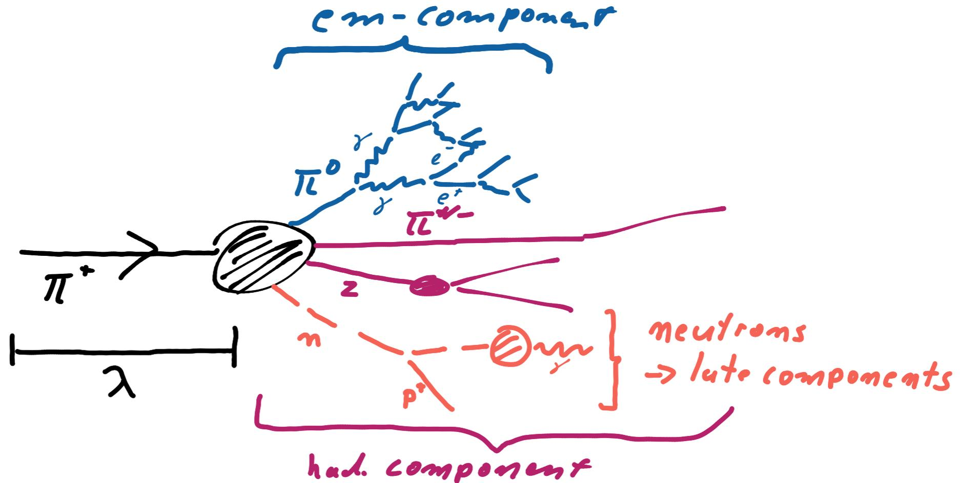
⇒ Granularity finer than typical shower structure can be exploited to improve the energy resolution
