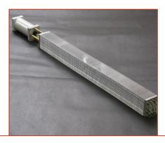
$\begin{array}{ll} \text{Dimensions} & 60\text{x}60 \text{ mm}^2 \\ \text{Radiation length} & 17 \text{ mm} \\ \text{Moliere radius} & 36 \text{ mm} \\ \text{Radiation thickness} & 25 \text{ } \text{X}_0 \\ \end{array}$
