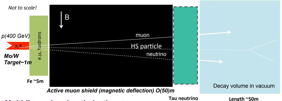
Multidimensional optimization: beam energy, Detector ~10m beam intensity, background conditions and detector acceptance Instrumentation Seminar, DESY
